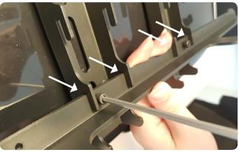
Loosen the threaded rods under the couch with an Umbraco key size 5. Do not screw the rods all the way out, but only until you can lift the top part 0,5-1 cm up.
