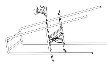
**4.** Remove the 8 screws from the top of the frame.
